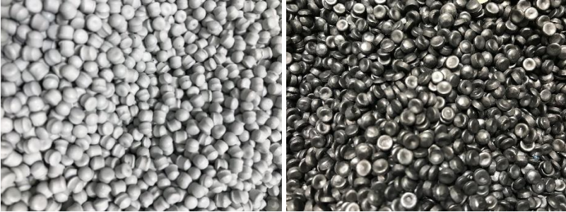
Figure 5: rPP regranulate (left: dark grey basic variant, right: black pigmented) © Öko-Institut/Andreas R. Köhler
